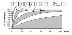
*Digital Filtering* module response to a temperature change. The illustration above demonstrates the effect of digital filtering (set with Filter Constant) on
